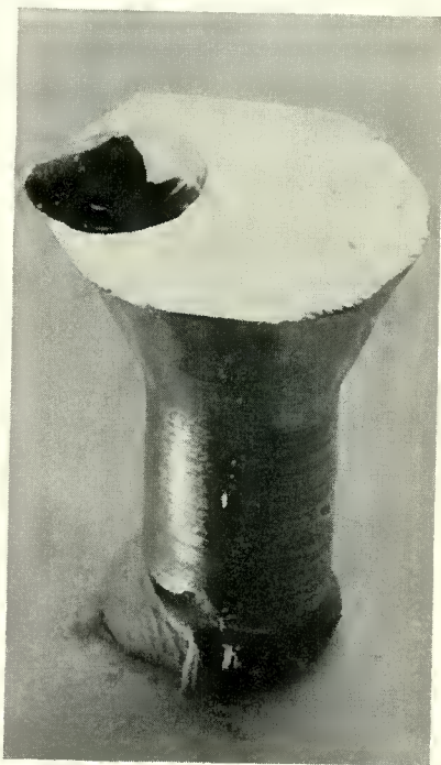
Fig. 11—Planar solid-liquid interface as revealed by rapid withdrawal of small diameter crystal from the melt. Conical protuberance is result of liquid drop retained by crystal surface on withdrawal. \times 3
