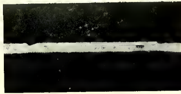
Fig. 4—Cross section of an alloyed junction (15 \times ). The p-n junction is crystallographically flat as defined by a {111} plane.
