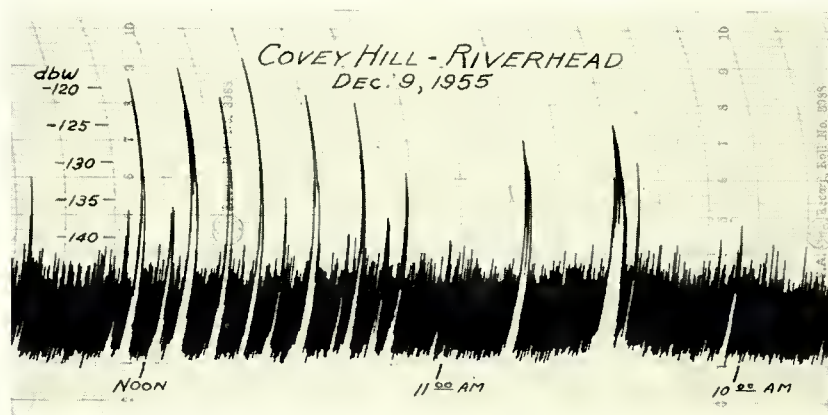
Fig. 8—Typical winter sample recording of received field strength. The large spikes were caused by aircraft reflections.
